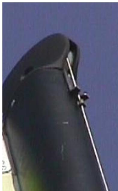
**3 When the sail is all the way up, pull the halyard forward sufficient for the stop sleeve to clear the halyard hook. Once the sleeve is past the hook, position the halyard so that the sleeve will engage the hook when you release tension. That done, secure the halyard to the mast cleat at the bottom of the mast and put the excess line in the tramp pocket with the jib halyard.**
