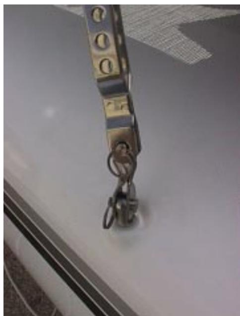
**6 Attach the wire shrouds in the fifth hole starting from the top of the shroud adjusters. Make sure the mast is held by the trapeze wires otherwise it will fall down.**
