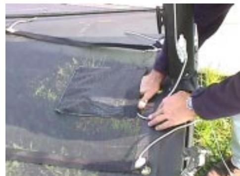
**Attach the upper block to the main hook and attach the hook into the middle hole of the main clew plate. Attach the ratchet block to the traveller car on the rear crossbar with the clevis pin and lock ring provided. Check that the two blocks are facing each other. Take the mainsheet, run the free end through the cam cleat of the ratchet block and tie a figure of eight knot to secure the line. Then the installation is as follows :**
